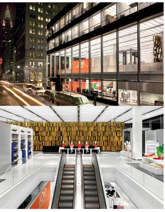
**Top:** Fluorescent ceiling fixtures glow behind acrylic panels, replacements identical to the originals. **Bottom:** Escalators were reoriented 90 degrees by SOM during the base-building
